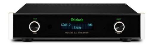
**FRONT PANEL:** Glass with LED/fiber-optic illuminated green nomenclature. INPUT/SETUP SELECTOR. IR SENSOR. Alphanumeric Fluorescent display with indicators for SOURCE selection, SAMPLING FREQUENCY, VOLUME level and SETUP mode selections. Standby indicator. ADJUST / STANDBY/ON control.
