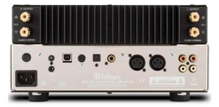
BACK PANEL: Gold plated Right channel OUTPUT terminals for 8 Ω speakers. Gold plated Left channel OUTPUT terminals for 8 Ω speakers. Fuse/Power cord receptacle.
