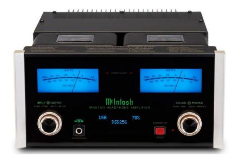
**FRONT PANEL:** LED/fiber-optic illuminated green nomenclature. Left POWER OUTPUT meter (LINEAR WATTS or DECIBELS). Left POWER GUARD light. IR sensor. Right POWER GUARD light. Right POWER OUTPUT meter (LINEAR WATTS or DECIBELS). SETUP / TRIM control. HEADPHONES jack. Digital information display. Pushbutton switch: STANDBY/ON / RESET (with indicator). Concentric VOLUME / PROFILE control.
