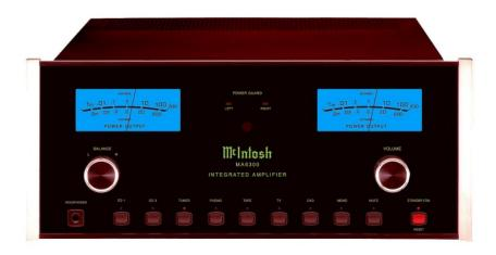
FRONT PANEL: Glass with LED/fiber-optic illuminated green/gold nomenclature. Left channel power output meter (LINEAR WATTS). LEFT POWER GUARD light. IR sensor. RIGHT POWER GUARD light. Right channel power output meter (LINEAR WATTS).
