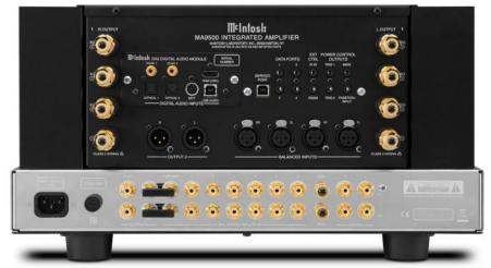
BACK PANEL: Right speaker OUTPUT connectors for 8, 4 and 2 OHMS. DA 2 DIGITAL AUDIO MODULE: DIGITAL AUDIO INPUTS: COAX 1, COAX 2, HDMI (ARC) / OPTICAL 1, OPTICAL 2, MCT, USB AUDIO. SERVICE PORT. DATA PORTS: 1, 2, 3, 4. EXTERNAL CONTROL: IR IN / RS232. POWER CONTROL OUTPUTS: TRIG 1 / TRIG 2, MAIN / PASSTHRU INPUT. Left speaker OUTPUT connectors for 8, 4 and 2 OHMS.
