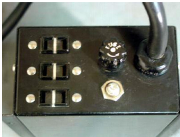
D 8A - Power supply for C 4 and C 8 preamplifier. Solid state. Replaced D 8.
