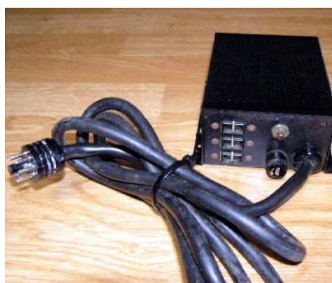
D 8 - Power supply for C 4 preamplifier. Tube: 5Y3GT
