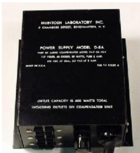
D 8A - Power supply for C 4 and C 8 preamplifier. Solid state. Replaced D 8.
