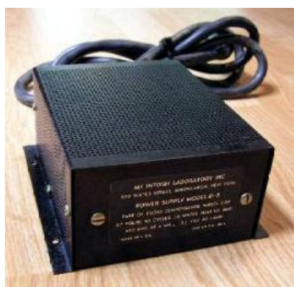
D 8 - Power supply for C 4 preamplifier. Tube: 5Y3GT
