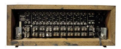
**REAR PANEL:** [Left and Right INPUT FROM SOURCE jacks. Left and Right TO **POWER AMP INPUT** jacks.  $\checkmark$  Left and Right **HOT TERM**inal spade connectors.  $\checkmark$ Left and Right COMmon TERMinal spade connectors.] / [Speaker 8 section: Left and Right jacks.  $\checkmark$  EQ: OUT or IN switch.  $\checkmark$  FROM / EQ jacks.  $\checkmark$ Right **TO SPEAKERS** spade connectors.] / [Speaker **7** section: Left and Right jacks. EQ: OUT or IN switch.
