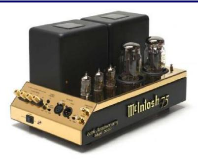
CONTROLS & CONNECTORS: Titanium gold plated stainless steel/black chassis. OUTPUT connectors for common, 2, 4 and 8 OHMS. POWER CONTROL jacks: IN / OUT. INPUT SENSITIVITY switch: 1.7V or .85V. BALANCED audio XLR INPUT jack, IN/OUTPUt jack. INPUT switch: BALanced or UNBALANCED audio INPUT / IN/OUTPUt jack. POWER switch OFF/ STandBY or ON. Standby/Power On and Sentry Monitor tube protection activation indicator.
