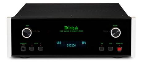
**FRONT PANEL:** Glass with LED/fiber-optic illuminated green nomenclature. INPUT / TRIM/SETUP MODE control. IR sensor. VOLUME / TRIM/SETUP control. jack. Touch buttons: OUTPUTS 1 and 2 (with indicators). Digital information display. Touch buttons: TONE (with indicator), MUTE, STANDBY/ON / RESET (with indicator).
