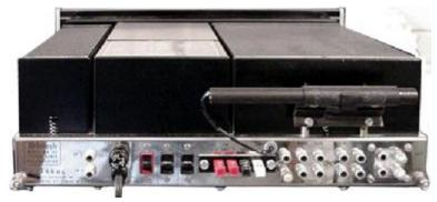
**BACK PANEL:** Scope outputs: TP 1 and TP 2. FUSE. Power cord. AC OUTLETS: 1 UNSWITCHED, 2 SWITCHED. Push terminals: AM ANT, GROUND, 300 OHM and 75 OHM ANTENNA. L+R OUTPUT. Ground terminal. OUTPUTS: MAIN, TAPE. INPUTS: AUX, TAPE, PH 1, PH 2. Panloc mounting.
