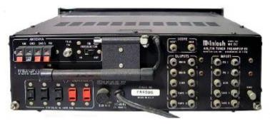
BACK PANEL: ANTENNA push terminals: AM, Ground, 300 Ω, FM. 75 Ω coaxial FM connector. FM PRESELECTOR switch: IN or OUT. Built-in ferrite antenna.
