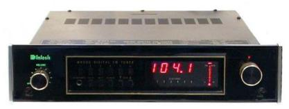
FRONT PANEL: Glass with illuminated teal/gold nomenclature. VOLUME with on-OFF switch. Push Buttons: 6 station presets. HEADPHONES jack. Push Buttons: ENTER, MUTE, MANUAL, SCAN ▲, SCAN ▼. Digital frequency readout. Indicator lights for 6 STATIONS presets. FM MPX light. LED column for signal strength. Tuning indicator: - ▲ or + Tuning control. PANLOC buttons.
