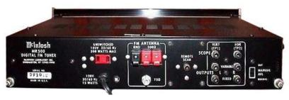
**BACK PANEL:** UNSWITCHED AC outlet. Power cord. Push terminals for: GND, 300  $\Omega$  FM ANTENNA. 75  $\Omega$  FM ANTENNA coax input. REMOTE control SCAN jack. SCOPE outputs: VERTical (TP1) and HORizontal (TP2). Audio OUTPUTS: Left & Right 2.5V VARIABLE and 1V FIXED. MANUAL AFL switch: OUT or NORMAL. Panloc mounting.
