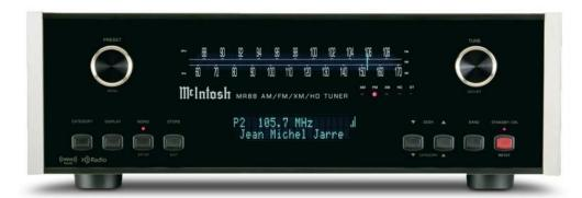
FRONT PANEL: Glass with LED/fiber-optic illuminated green/gold nomenclature. IR remote sensor. PRESET / MENU control. Dial glass with electronic tuning pointer. Indicators for AM, FM, XM, HD, STEREO reception. TUNE / ADJUST control.
